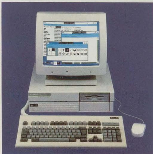
**BULL MICRAL - 200:** RAM 1 MB - DISCO FIJO 20 MB - DISKETTE 1,44 MB 3 1/2" - MONITOR VGA - SIST. OPERAT. MS/DOS
